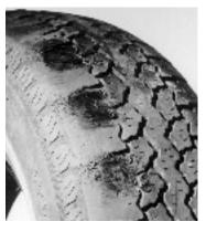
when the vehicle suspension loses its ability to absorb "jounce travel." "Jounce travel" is the upward movement of the tire in relation to the vehicle's downward movement. This condition most commonly occurs with weak shock absorbers or incorrect shock application.
