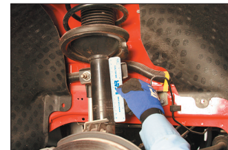
Figure 5– Small straightedges can be used to check for a bent strut cartridge.
